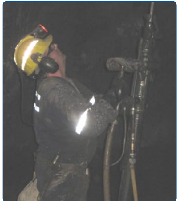
Figure 4: Operating a Stoper to Drill Hole Overhead
