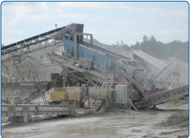
Figure 3: Portable Conveyors and Screen
