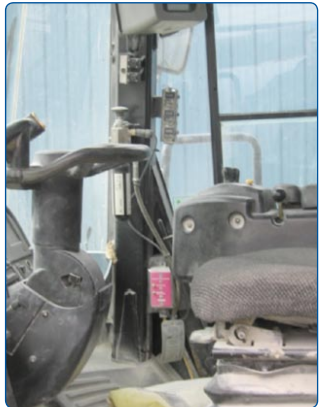
Figure 4: Controls inside a loader
